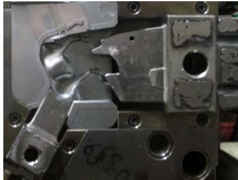
Injection Side of the Two Cavity Mould
