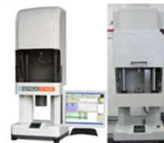
CR-6000 Capillary viscosity at different temperature and shear rates pvT-6000 pvT change at different temperature and pressure
